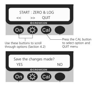
Press the first button to save the change and move the menu back up a level, and the last key to leave the selection as it was (unchanged) and move back up a level.
